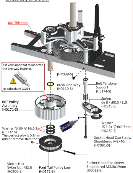
Position without preload. Insert the screw in the hole through the aluminum support as in the picture.
