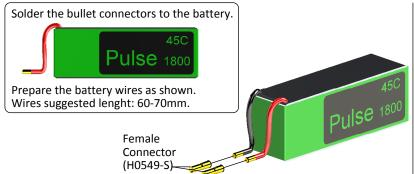
Insert the bullet connectors in the plastic housing, you can apply a little heat to the plastic to facilitate the insertion.
