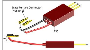
Solder the two bullet connectors (H0549) as shown. Try to solder the wires with the least amount of vertical dimension (Z).
