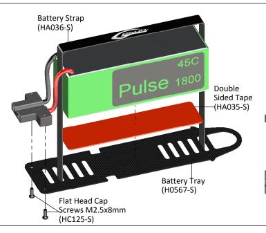
Mount the battery to the tray using double sided tape and the long Velcro straps included.
