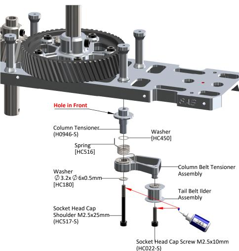
Move the tail case and tighten the belt until the tensioner is in this position.
