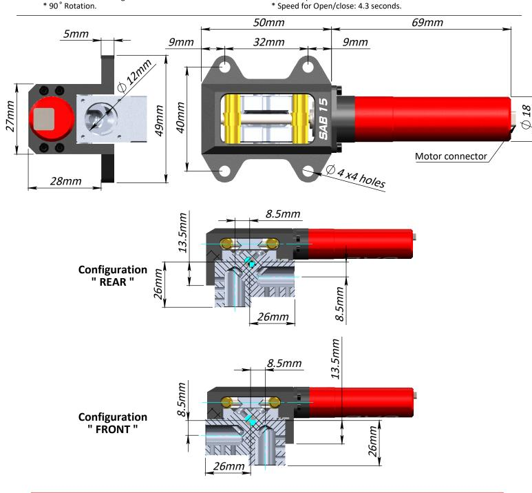
The motor blocked at maximum current may be damaged. Use an appropriate control unit with limitation/stop current.
