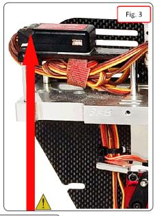
It is important to lock the plugs of the flybarless unit with an adhesive - for example hot glue.
