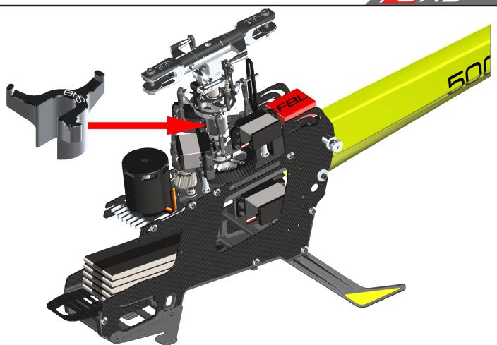
The swashplate leveler allows you to locate the center position for the swashplate and to verify that it is horizontal. It is used in the calibration step and thanks to it's design, it allows you to quickly check your setup without removing the head.
